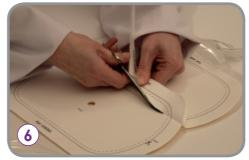
Position the pouches so the release paper is facing up. Cut the peeled back release paper away.
